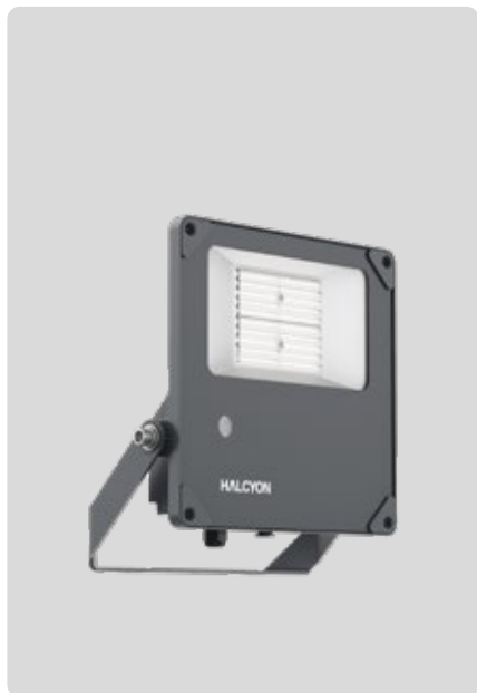
X500 <50W Dimensions L342 x W310 x D56mm Watts Selectable 25W, 37.5W or 50W Lumens <7100lm Beam 90° x 60°
