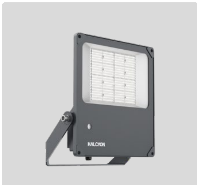
X503 <200W Dimensions L474 x W410 x D61mm Watts Selectable 100W, 150W or 200W Lumens <29200lm Beam 90° x 60°
