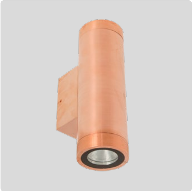
EX112Two Way Overall Dimensions L190 x W47 x D89mm Beam 2x 45° Watts 2x 5W Lumens 2x 350lm
