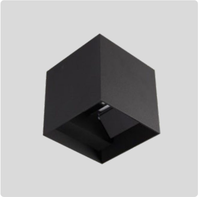
EX919 Medium Dimensions L120 x W120 x H120mm Lumens <935lm Watts 11W Beam Adjustable 0 - 120°
