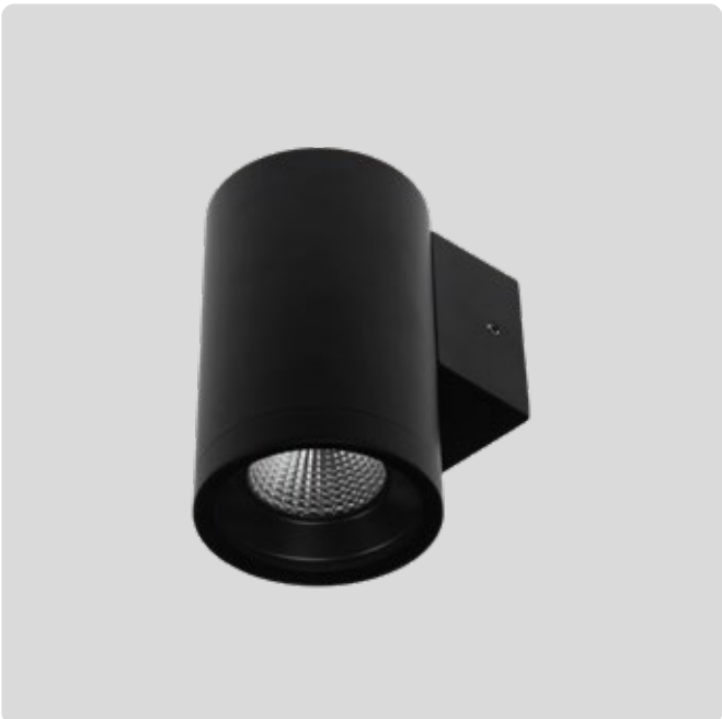
EX152 Large One Way (Up or Down)* Dimensions L160 x W110 x H155mm Beam 40° Watts 18W Lumens 1800lm
