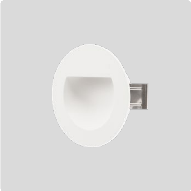
EX900 Round Dimensions D90 x H36mm Beam 120° Watts 3W Lumens <95lm Cut Out Ø 72mm (Ø 76mm if using housing)
