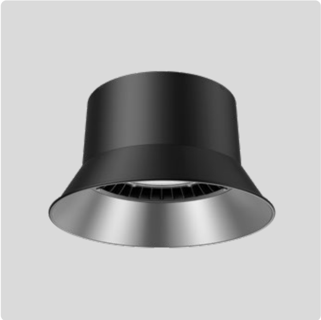
P301 Mid/Low Bay Dimensions Ø393mm x H286mm Beam 90° Watts Selectable 90W, 120W or 150W Lumens <17,000lm
