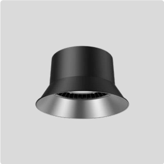
P300 Low Bay Dimensions Ø264mm x H231mm Beam 90° Watts Selectable 42W, 56W or 70W Lumens <7915lm
