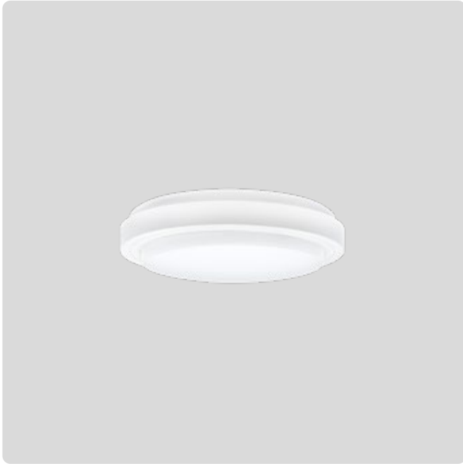
LED290 Small Dimensions D200 x H43mm Beam 110° Watts Selectable 10W or 15W Lumens <1650lm
