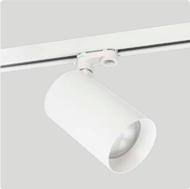
S217 Large Spot Ø110mm x L185mm Lumens <2200lm Watts 20W Tilt 90° Rotate 360° Beam 38°
