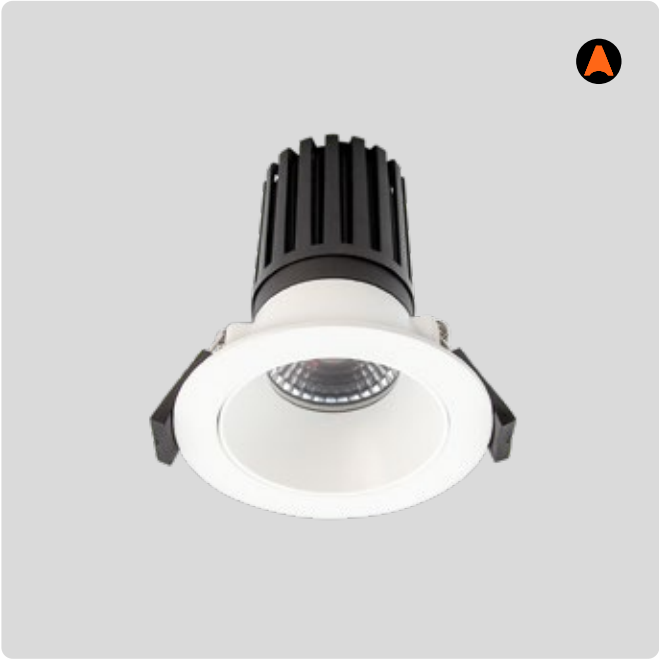
R730 R731 Small Dimensions D93 x H104mm Cut Out Ø 72-82mm Watts 9.5W Lumens <930lm Beam 50° or 90°
