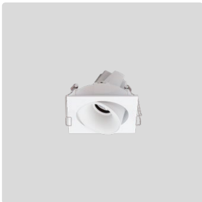
R550 Small Dimensions L86 x W86 x H66mm Cut Out Ø 80mm Watts 11W Lumens 740lm Beam 40° Tilt 25° Rotate 355°
