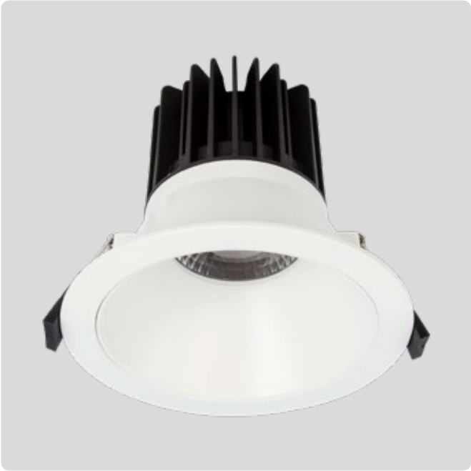
R602 R603 Large Selectable Wattage Dimensions D150 x H130mm Cut Out Ø 130-140mm Watts Selectable Lumens <1870lm Beam 60° or 90°
