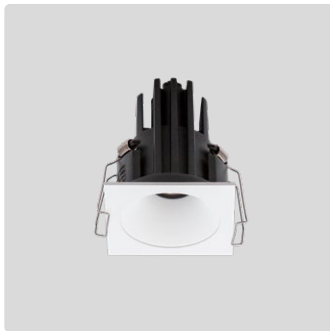
R541 Small Dimensions L65 x W65 x H72mm Cut Out Ø 60mm Watts 11W Lumens <685lm Beam 60°
