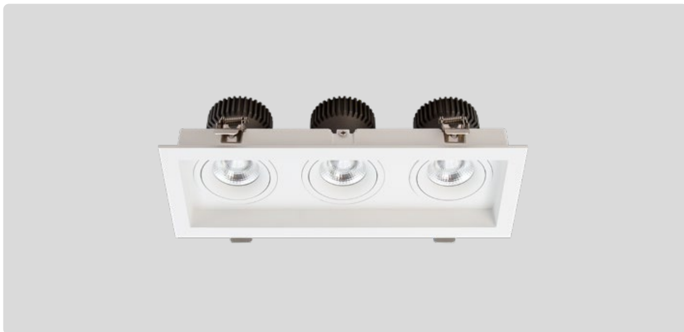
R513 Triple Dimensions L300 x W115 x H95mm Cut Out L280 x W95mm Watts 3x 11W Lumens 2730lm Beam 3x 50° Tilt 30° Rotate 358°
