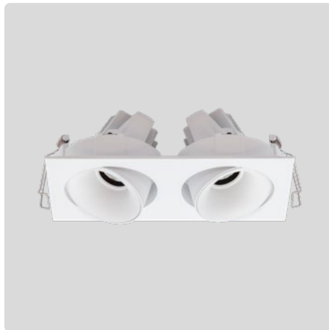
R551 Small Double Dimensions L170 x W86 x H65mm Cut Out 165 x 80mm Watts 2x 11W Lumens 2x 740lm Beam 40° Tilt 25° Rotate 355°
