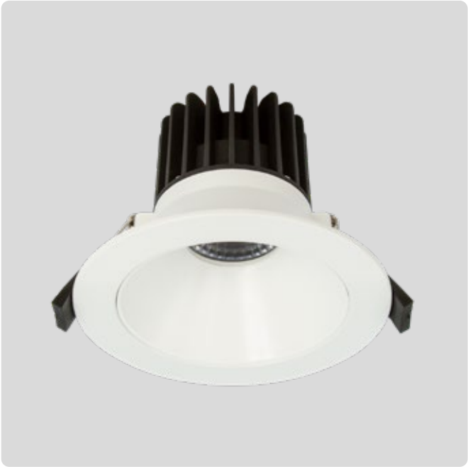
R610 R611 Medium Dimensions D126 x H95mm Cut Out Ø 100-110mm Watts 12W Lumens <950lm Beam 50° or 90°
