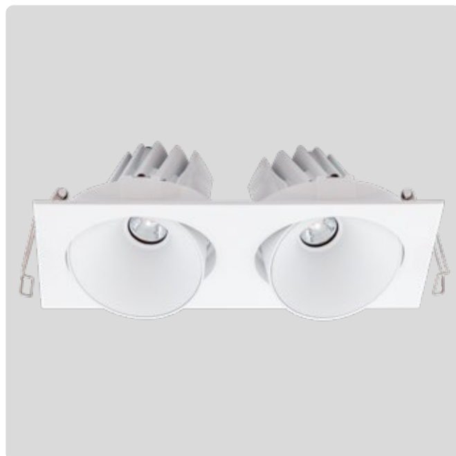
R554 Medium Double Dimensions L215 x W105 x H82mm Cut Out 205 x 100mm Watts 2x 14W Lumens 2x 1000lm Beam 40° Tilt 32° Rotate 355°
