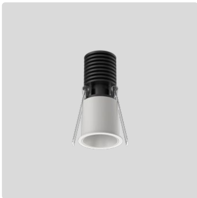
R534 Mini Dimensions D46 x H105mm Cut Out Ø 40mm Watts Selectable 4.3W, 5.4W, 6.5W or 8W Lumens <580lm Beam 24°
