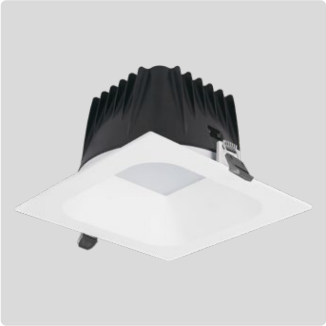
R743 Large Dimensions L212 x W212 x H120mm Cut Out Ø200mm Watts 26W Lumens <3030lm Beam 70°
