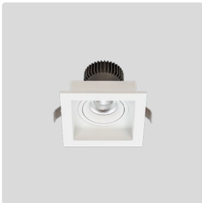
R511 Single Dimensions L115 x W115 x H95mm Cut Out L95 x W95mm Watts 11W Lumens 983lm Beam 50° Tilt 30° Rotate 358°
