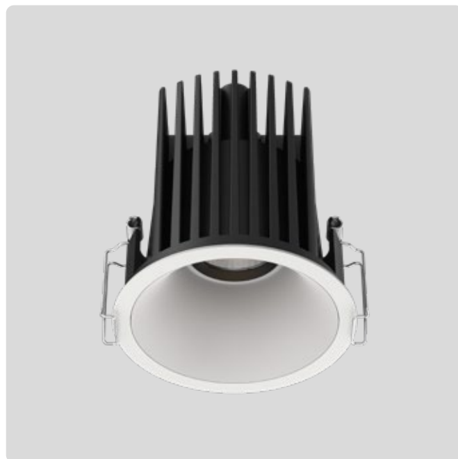
R537 Large Dimensions D106 x H110mm Cut Out Ø 100mm Watts 20W Lumens <1480lm Beam 40°
