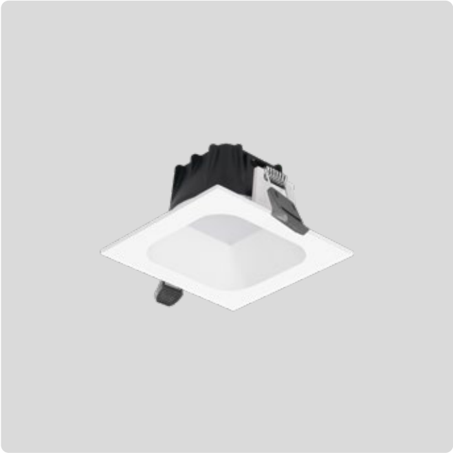
R741 Small Dimensions L100 x W100 x D52mm Cut Out Ø90mm Watts 10W Lumens <1190lm Beam 75°
