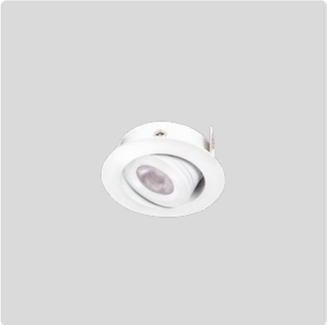
R782 Semi Narrow Beam Tilt Dimensions D52 x H25mm Cut Out Ø 46mm Watts 3W Lumens 120lm Beam 36° Tilt 30°
