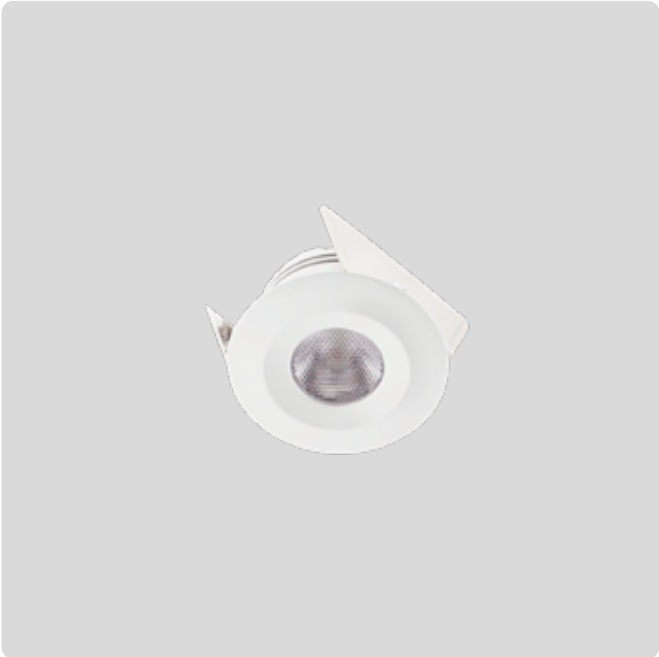
R781 Semi Narrow Beam Fixed Dimensions D41 x H21mm Cut Out Ø 37mm Watts 3W Lumens 120lm Beam 36°
