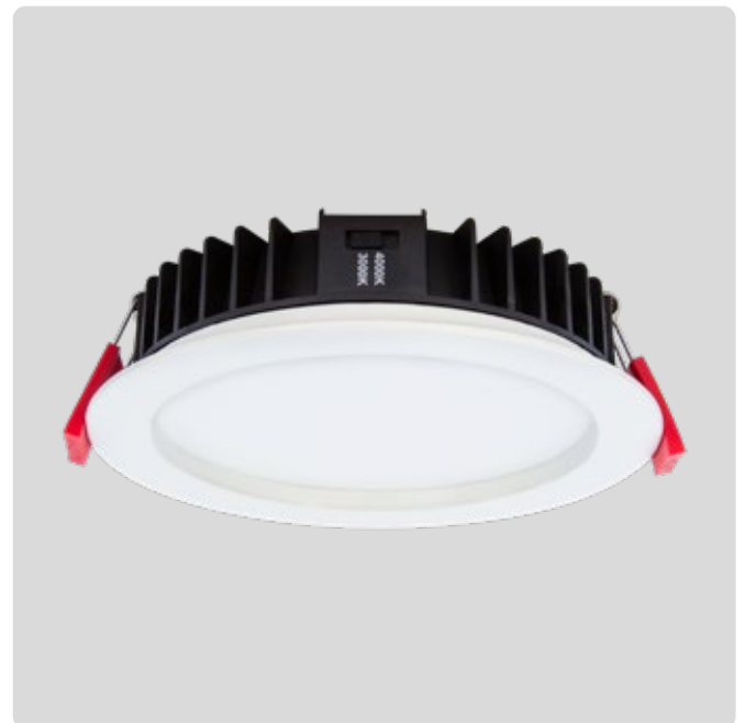
R774 Large Fixed Dimensions D160 x H43mm Watts Selectable 9W or 15W Beam 100° Cut Out Ø 145mm Lumens <1950lm
